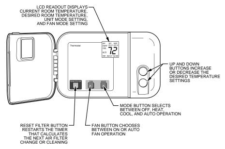
Fig. 2—Carrier Non-Programmable Thermostat
